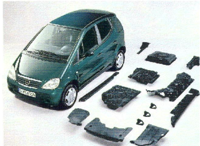
**Figure1: Car Interiors from Natural Fiber – Polypropylene Composites**
