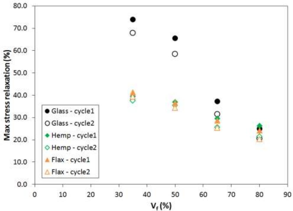
Figure 4: Evolution of the maximum stress relaxation with fibre volume fraction. The results were very reproducible with less than 3% of standard deviation measured for each reinforcement
