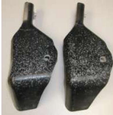
Figure 5: Prototype underbody shields using vinyl ester resin (L) and soy resin (R), after stone impact gravelometer testing
