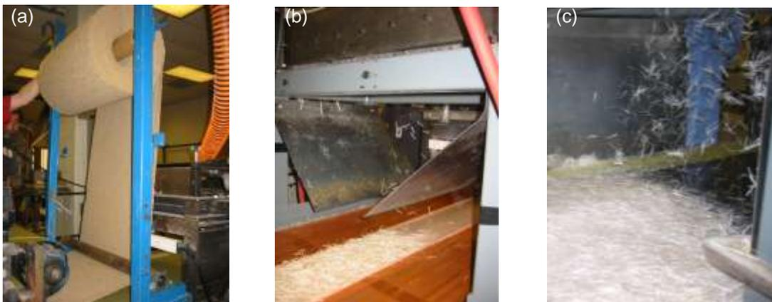
Figure 1. Continuous SMC compounding line utilizing: (a) non-woven hemp mat; (b) chopped hemp twine; and (c) hybrid mixture of chopped hemp twine and glass.
