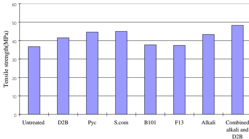
Figure 8: Tensile strength of untreated and treated fibres composites
