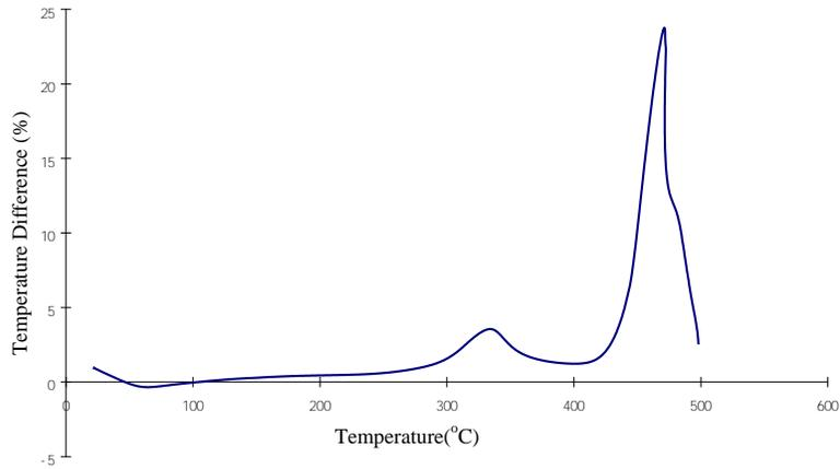
Figure 5: DTA curve of untreated fibre
