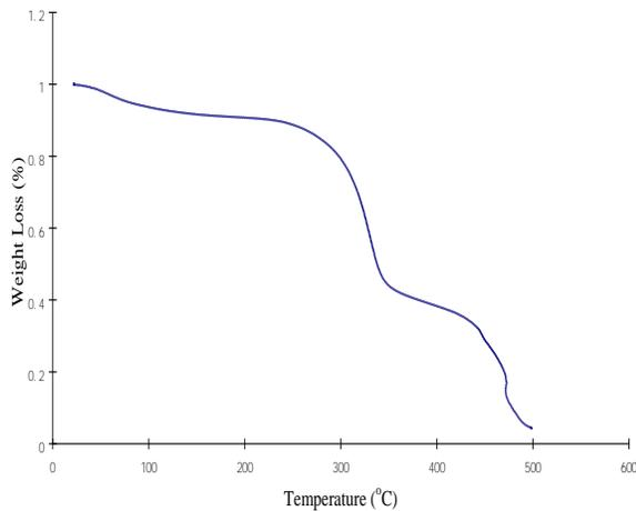
Figure 6: TGA curve of untreated fibre
