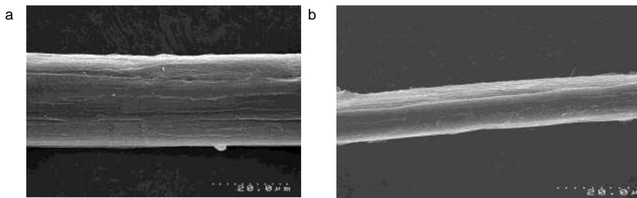
Figure 2: SEM micrographs of fibre treated with a) alkali, b) D2B fungi
