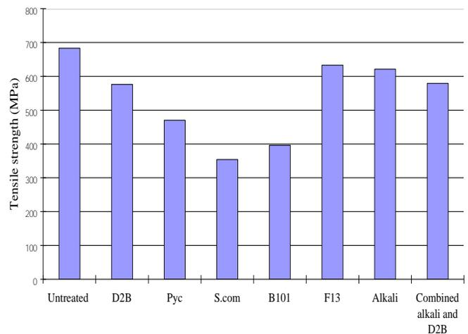
Figure 7: Single fibre strength
