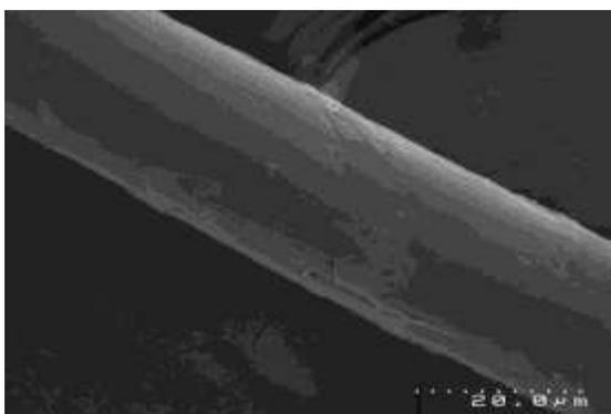
Figure 1: SEM of untreated hemp fibre
