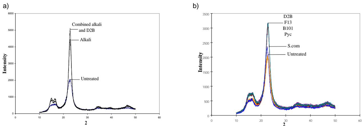
Figure 4: X-Ray Diffraction Traces for a) untreated, alkali treated and combined alkali and D2B treated fibre, b) untreated and fungal treated fibres(y-axis expanded compared to a)
